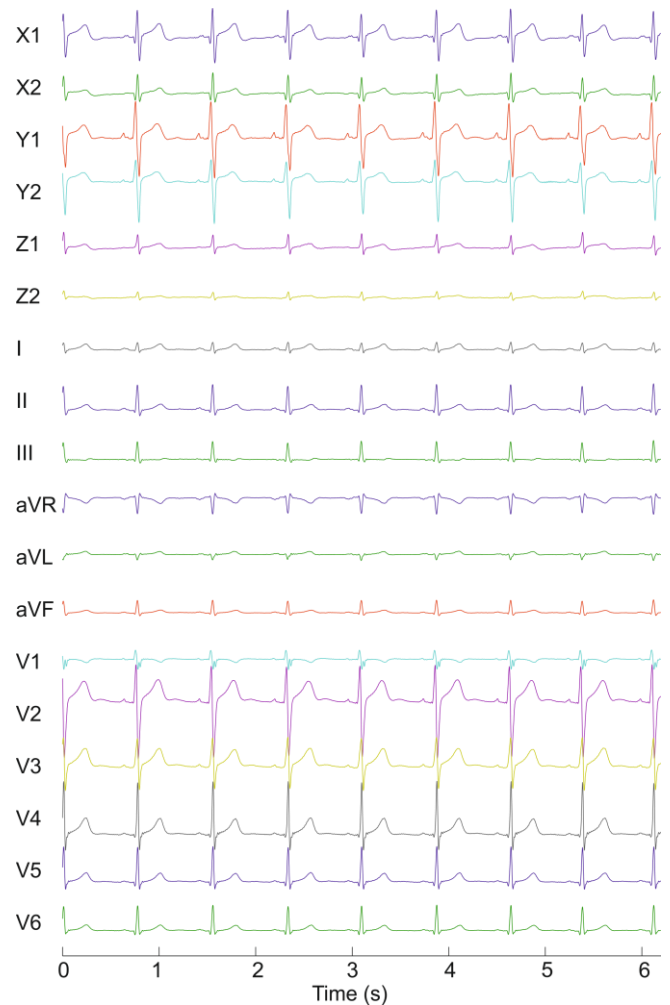
Figure 15. Illustration of ECG example from the three ePatch ECG recorders and the standard 12-lead ECG equipment. The top six traces illustrate the two channels from each of the three ePatch sensors, and the lower 12 traces illustrate the traditional 12-lead ECG. A high similarity is observed between Y1 and V2.
