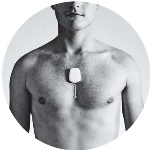
Figure 2: Illustration of the placement of the ePatch electrode and sensor on the sternum.
