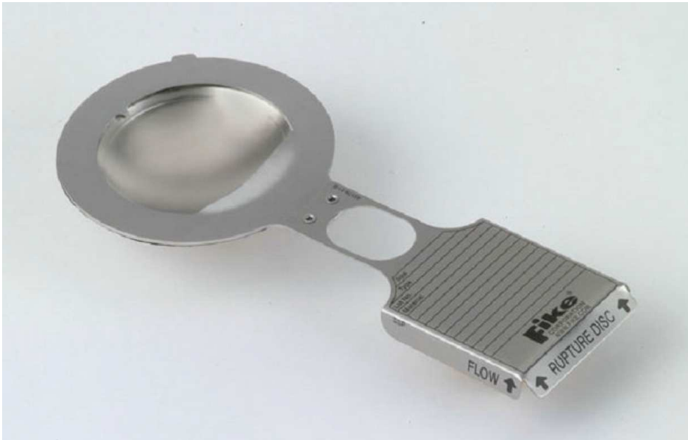
Figure 5 Reverse buckling type rupture disc (dome points towards the fluid pressure) similar to the one installed on the incident storage tank. Proper flow direction of pressure release is marked on the nameplate (Photo courtesy: Fike®)
