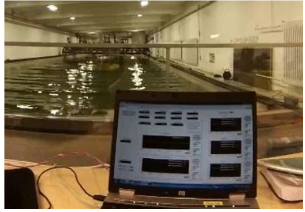
Fig. 4. Operator laptop where DP setpoints and controller gains are specified. The wave flap is also seen directly behind the laptop.
