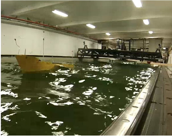
Fig. 2. Cybership 3 in action. The three cameras measuring position are seen above the bridge structure, and the surface elevation is measured to the far right at the wooden plank.
