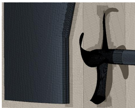
Figure 3. Computational mesh around the reference propeller and rudder
