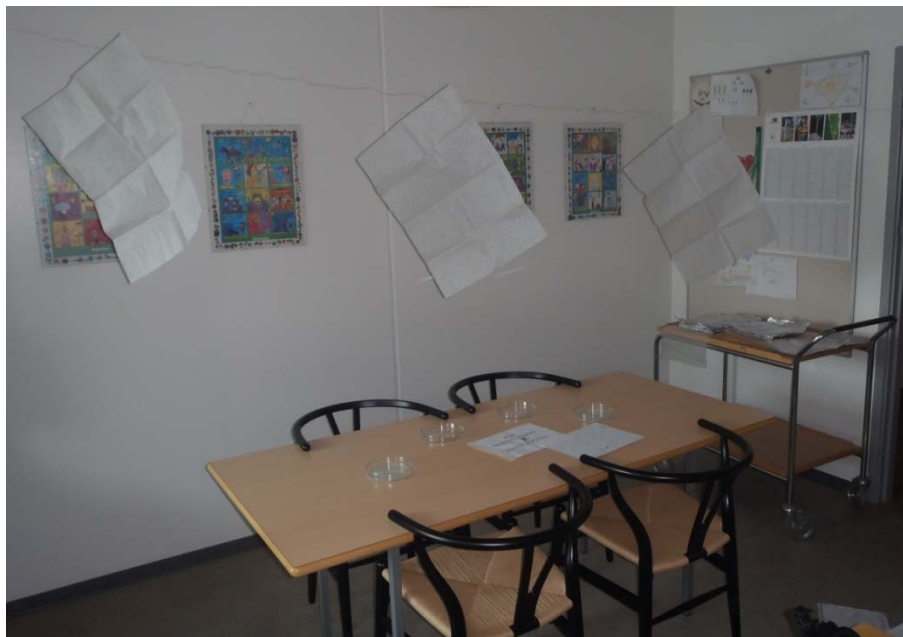
Figure 21. Example of a passive sampling set-up. For quality assurance purposes, the sampling campaign included several replicates of petri-dishes and silicone-coated paper. Photograph taken by Rambøll.
