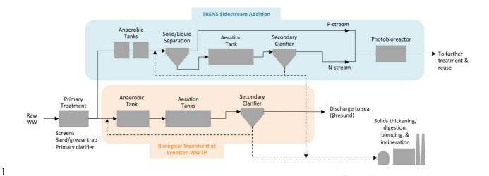
**Figure 1**: Flow diagram of TRENS system (EBP2R and downstream PBR) implemented as sidestream process to the existing Lynetten WWTP. Figure created from TRENS (Valverde-Pérezet al., 2014; Valverde-Pérezet al., 2015) and Lynetten process flow diagrams (Lynettefællesskabet I/S, 2012). Solid lines show flow of water, dotted lines show sludge or solids flow.
