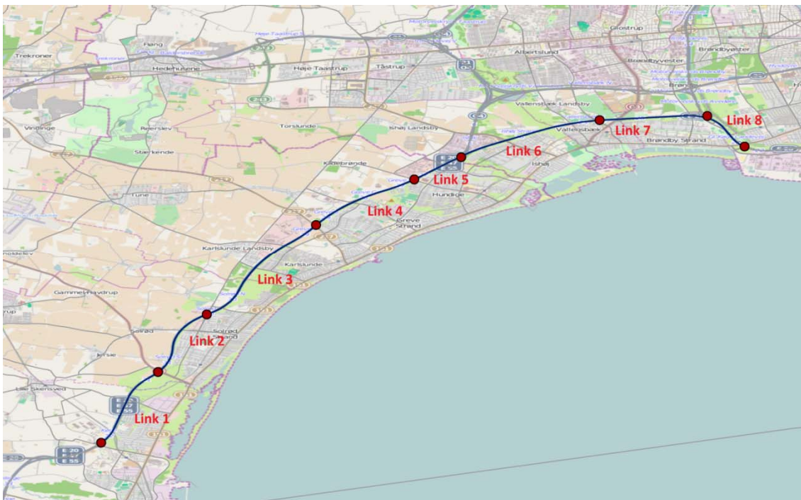
Figure 1: The eight road segments (links) on the Køge Bugt Motorway, separated by red dots. We consider the direction towards Copenhagen, i.e. from South-West towards North-East.
