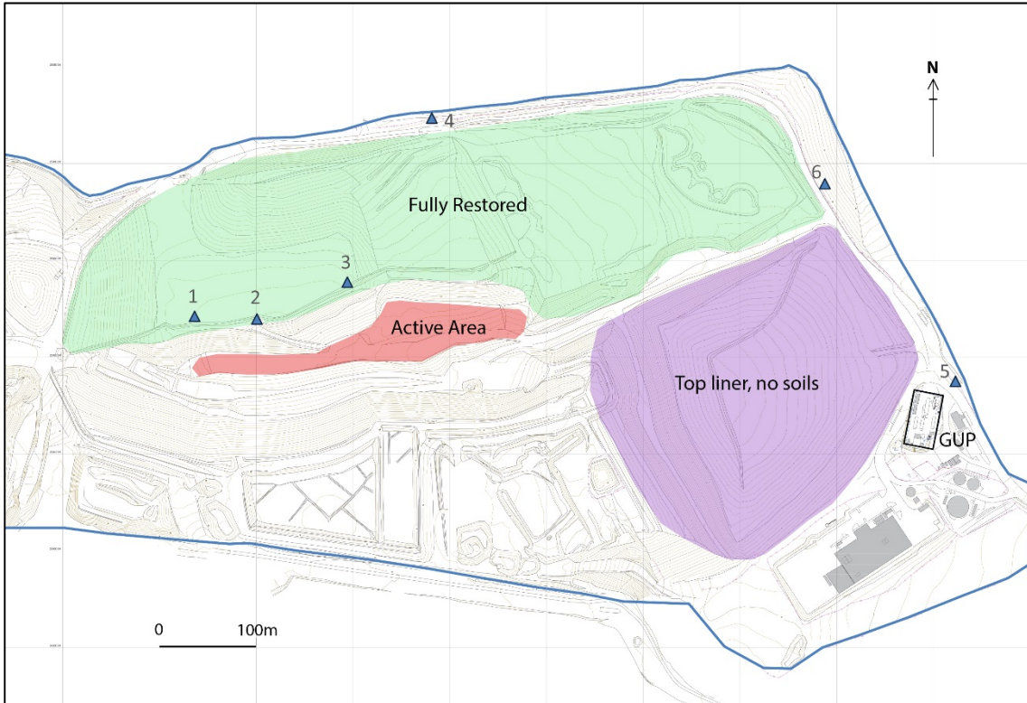
Figure 5. Plan of landfill showing location of the tracer gas bottles.
