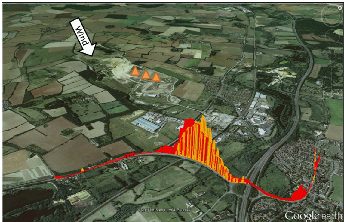
Figure 8. Three tracer gas bottles on Masons landfill (yellow triangles) and the downwind plume of methane (red) and tracer gas (yellow) 1600-1700 m away. Measurements were made on June 11 th , 2014. Maximum methane and tracer gas concentrations were approximately 400 and 2.2 ppb above background, respectively.
