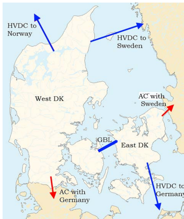
Figure 1: Danish power system interconnections with Nordic and CE power systems; Red lines indicate the AC connection and the Blue lines indicate the HVDC connection.
