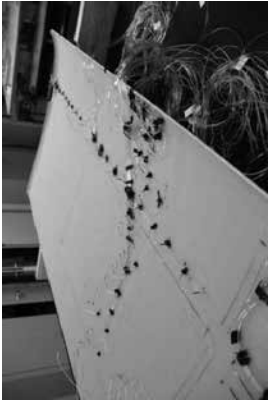
Figure 13 – Pressure taps installed on the suction side at the mid span position and along the span at 25% chord from the leading edge.
