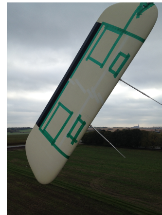
Fig. 2. The wing section with the flap mounted on the rotating rig test stand
