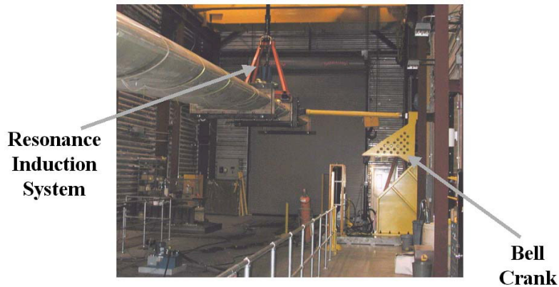
Figure 6: NREL's B-REX test System [8].
