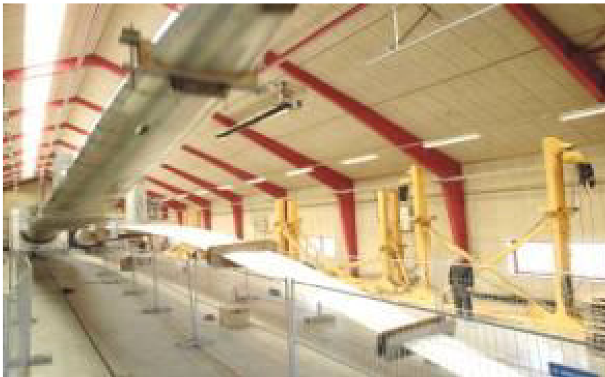
Figure 2: Flapwise fatigue test (courtesy of Blaest)
