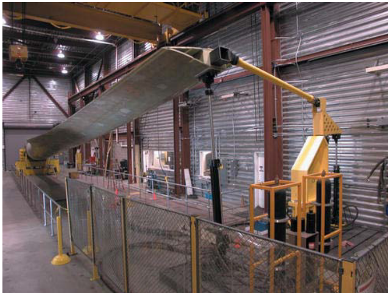
Figure 4: NREL's Dual Axis Force Displacement fatigue test [7].
