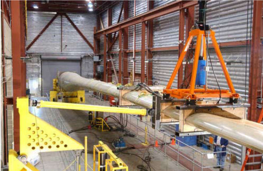
Figure 10: NREL's Hybrid System B-REX [8].
