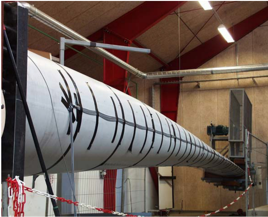
Figure 1: Fatigue test with single axis mass resonance using rotating mass test (courtesy of Blaest).
