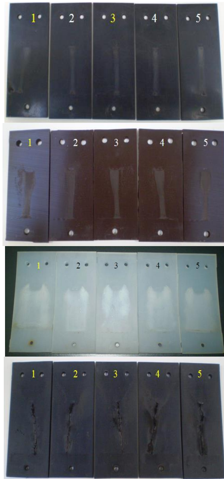
Figure 6-5. Surface erosion on the samples of the rubber materials after the tracking resistance tests. From top to bottom: Santoprene: Samples 1 and 3 failed, Silicone rubber: Sample 1 failed, PUR: Sample 1 failed, and EPDM: All the samples failed.
