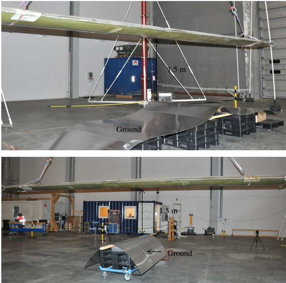
Figure 4-15. Blade section test setup, where the specimen is hanging at 1.5m from a ground plane. Above, setup for positive polarity. Below, setup for negative polarity.
