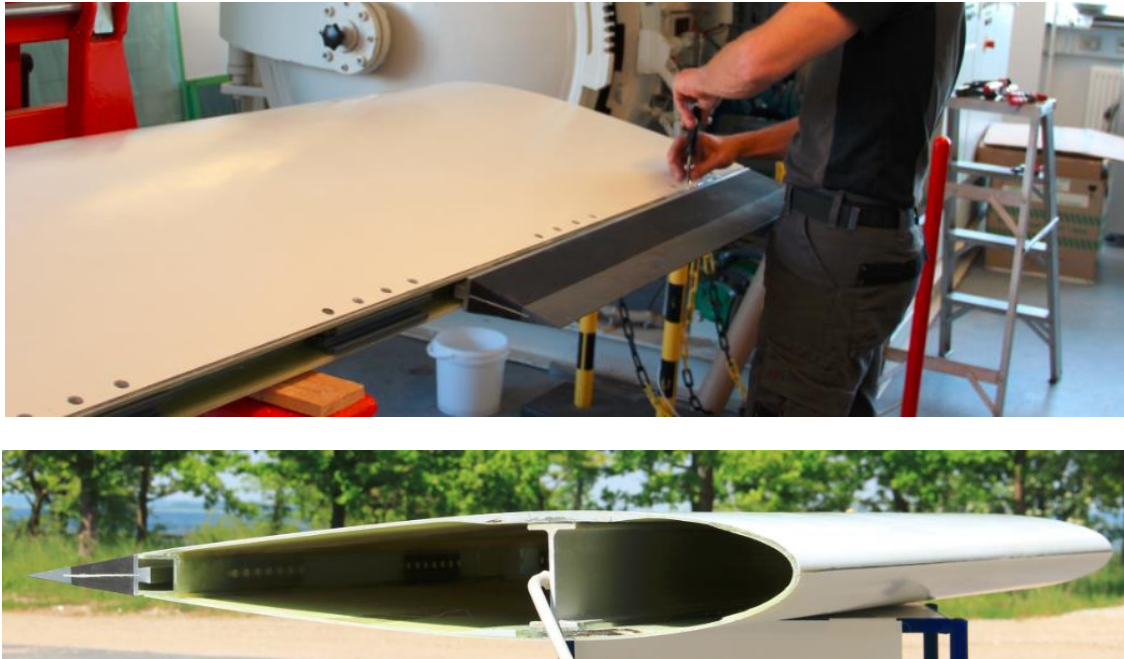
Figure 7-7. Prototype manufactured for testing. On the top, assembling of the rubber flap at the trailing edge using non-conductive bolts. On the bottom, finished prototype with the flap voids filled with propylene glycol.
