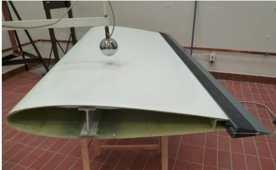
Figure 7-10. Setup of the high voltage swept channel tests performed to the prototype equipped with trailing edge flap and lightning protection system.
