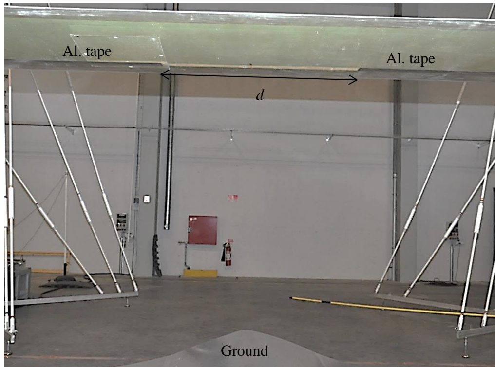
Figure 4-16. Aluminum tape stuck on the shell surface. Part of the tape is removed in a length d , over the protrusion on the grounding plane.
