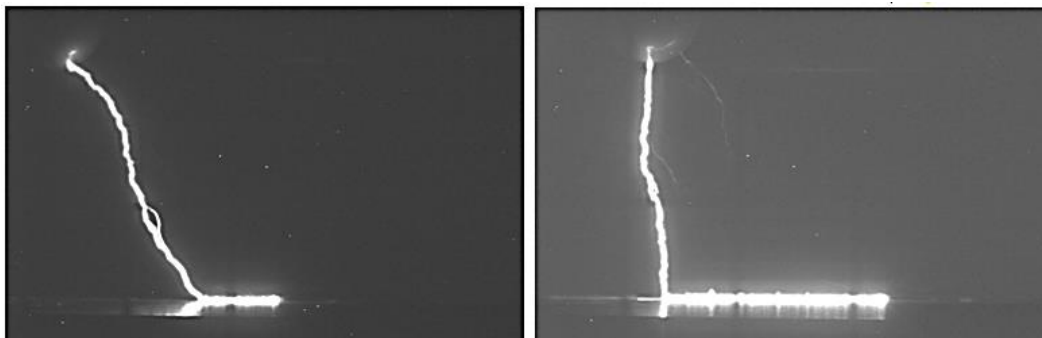
Figure 4-8. On the left, positive discharge in setup 1: the discharge path follows the panel surface approximately 100 mm. On the right, positive discharge in setup 3: The discharge path follows the panel 300 mm, the entire distance between the HV electrode and the receptor.
