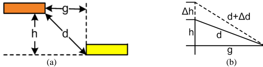
Fig. 2. (a) Cross section view illustration of two capacitively coupled electrodes on cantilevers; (b) extracted model for analyzing cantilevers deflection.
