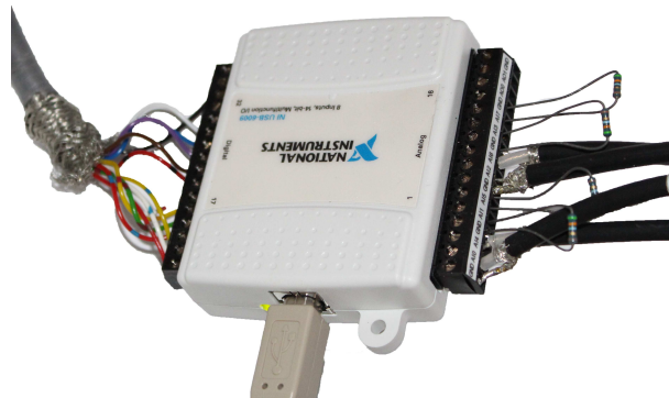
Figure 6.23: A photograph of the USB-6009 data acquisition module from NI.
