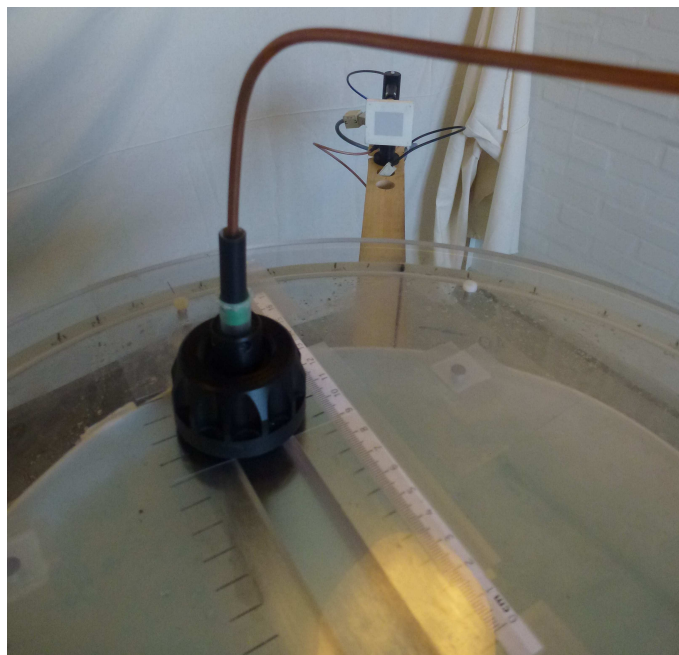
Figure 6.31: A photo of the internal antenna mount on top of the lid of the phantom. The slot where the internal antenna moves along is also seen with a ruler that indicates the distance offset from the centre of the phantom.
