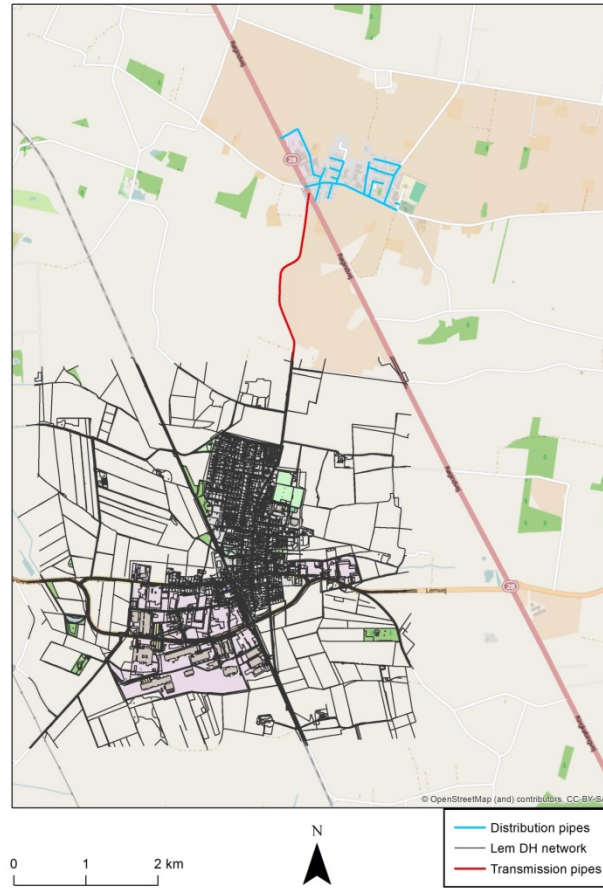
Figure 6. District heating network in Lem and assumed transmission and distribution district heating pipes
