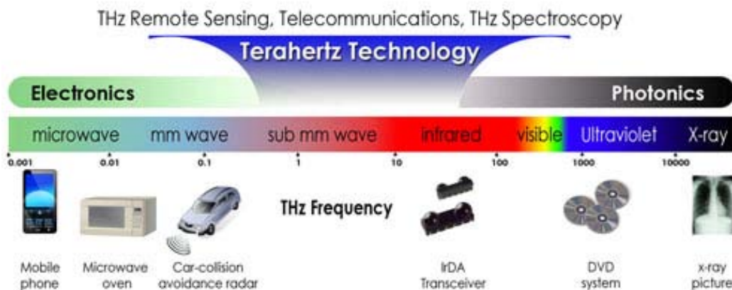
Figure 1.1 The electromagnetic spectrum, red region represent THz band in the electromagnetic spectrum.
