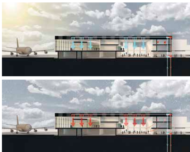
Figure 40 - Copenhagen Airport ATES system provide cooling in the summer (top) and heating in the winter (bottom).
