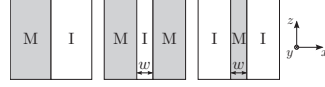
FIG. 1. The three waveguide systems: metal-insulator (MI), metal-insulator-metal (MIM), and insulator-metal-insulator (IMI) along with the chosen coordinate system.
