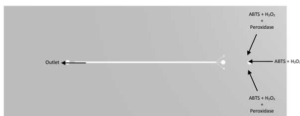
Figure 5.23 –Top view of the microchannel for the Five-stream microreactor.
