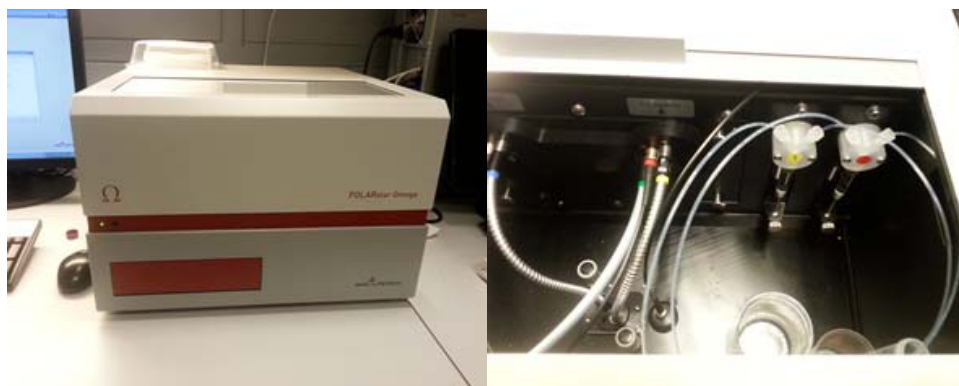
Figure B-1 - a) Microwell plate reader POLARstar from BMG LABTECH, b) Reactants compartment with two syringe pumps.
