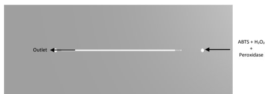
Figure 5.21 – Top view of the microchannel for the T-microreactor.
