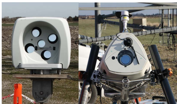
Figure 1. Wind profiling lidar examples: 5-beam AventLidar Demonstrator (left) and ZephIR DM (right)
