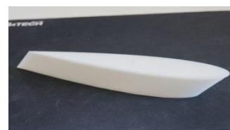
Fig. 2 Airfoil's blade produced on 3D printed with precision of 0.3mm (layer height)
