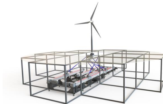
Fig. 1 Assembly of the nacelle of a Multi-Megawatt wind turbine scaled model (1/75).
