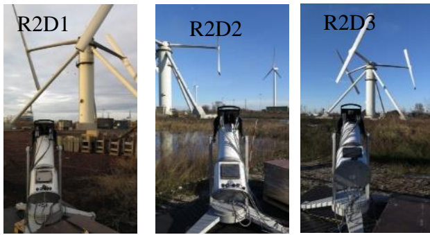
Fig. 1 Short-range WindScanners in operation around Nenuphar VAWT at Fos-sur-Mer, Fr.
