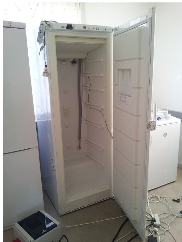
Figure 1: The 333 liters domestic freezer used for the identification and MPC experiments.
