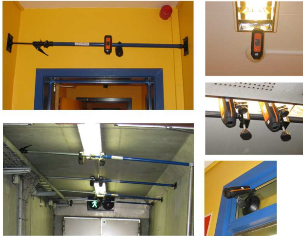
Figure 2.1: Mounting options for cameras using suction cups, clamps and moveable bars with pipe clamps.
