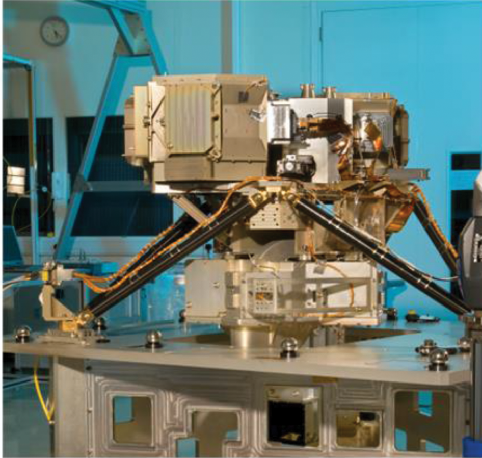
Fig. 1.— The MIRI Flight Model prior to delivery. The optics module structure is aluminium, and it is mounted to JWST with a (black) CFRP hexapod truss..
