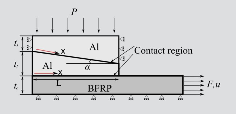
By optimizing the geometry it is possible to achieve as uniform as possible pressure distribution, while at the same time allowing the wedges to further slide and increase pullout force.
