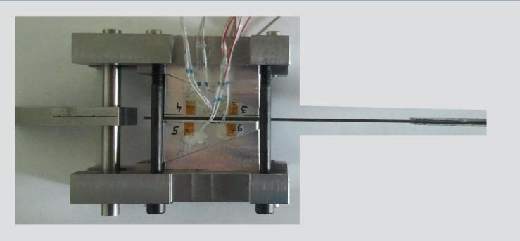
A test rig is used for model validation. Several wedge configurations can be tested and compared compared to numerical results. Pre-clamping pressure and strain levels can be monitored during the test. Preliminary test results have achieved pullout values lower the ones estimated with the FE model.
