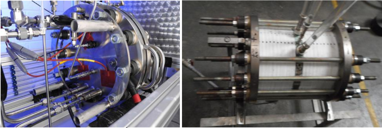
Figure 11: Single cell with 300 cm 2 electrodes size for testing the e-bypass-separator concept (left); 20 cell stack 10 kW range equipped with e-bypass-separators and VPS-coated electrodes (right)
