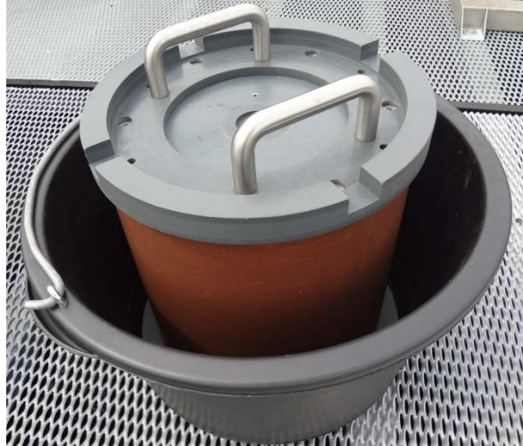
Figure 13A. Cylinder with grips attached to one end which was used to move the coated cylinder.
