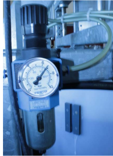
Figure 21A. Compressed air pressure reading equipment which is located on the left part of the frame setup.
