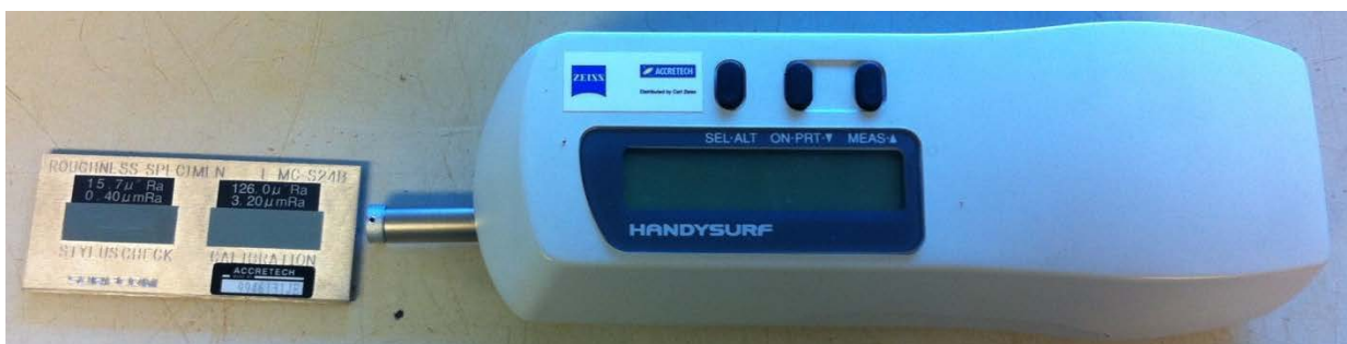
Figure 45A. The surfaces used to calibrate the equipment (left side) and the Handy-surf E350 (right side).
