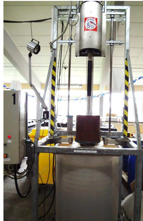
Figure 2.4. Laboratory rotor with a coated cylinder detached from the shaft.
