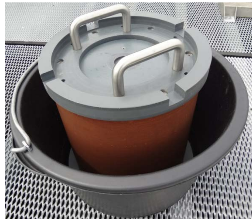
Figure 40A. Bucket to transport cylinder that could be filled with seawater to preserve biofouling.
