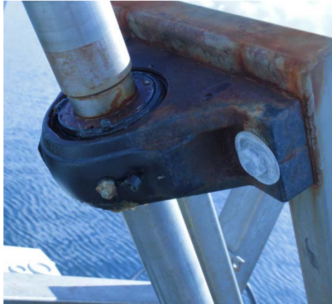
Figure 33A. One of two bearings at the dynamic rotor setup.
