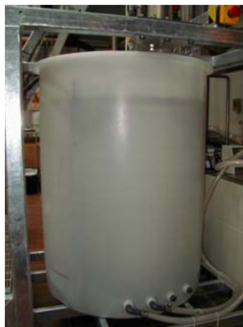
Figure 19A. The 580 l polypropylene tank.
