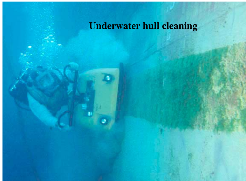
Figure 25.1. Example of an underwater hull cleaning with a rotating brush system, operated by a diver (modified from Bohlander and Zealand (2009)).
