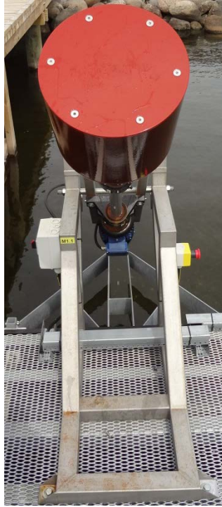
Figure 29A. Frame bolted to the raft. Two screws are seen on the ends of the stick going horizontally through the frame which ensured that the cylinder could flip out of the water.
