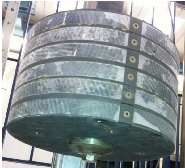
Figure 18A. Rotor cylinder with plastic strips attached. Mounting of the cylinder with strips is done by tightening the screw after the cylinder has passed through the shaft.
