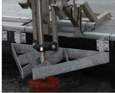
Figure 41A. Triangular frame protecting the coated cylinders from floating objects.
