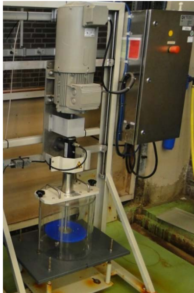
Figure 1.3. Friction disk machine used to measure the drag of coated disks, located at TNO, the Netherlands. Here shown with a blue disk in the chamber, which can hold water (here without water) (Klijnstra, 2014).
