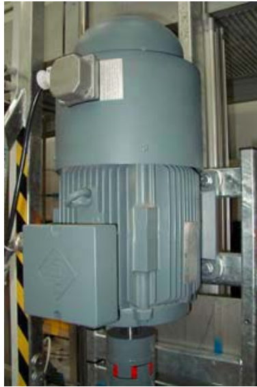
Figure 3A. The 7.5 kW engine used to rotate the cylinder in the tank and the additional cooling on top of the engine.
