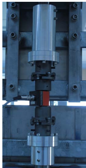
Figure 5A. Torque sensor and mounting system to the shaft. The wire is connected to the computer, which records the torque picked up by the torque sensor.
