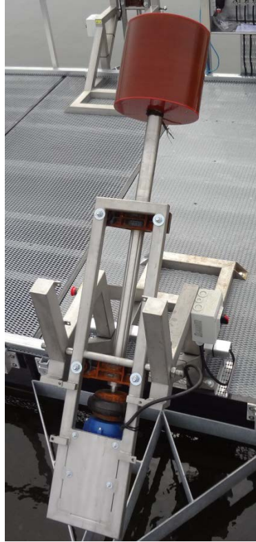
Figure 32A. Shaft, which was attached to the engine, going through two bearings and connected to a cylinder.
