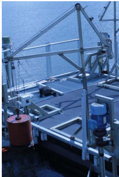
Figure 43A. Static immersion test setup at the raft with a cylinder lifted up from the seawater.
