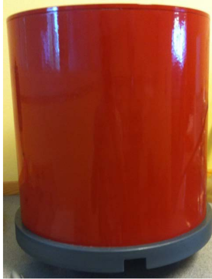
Figure 11A. Coated cylinder. The grips used to attach and dismantle cylinders from the laboratory rotor and aging setup are seen at the bottom of the cylinder.
