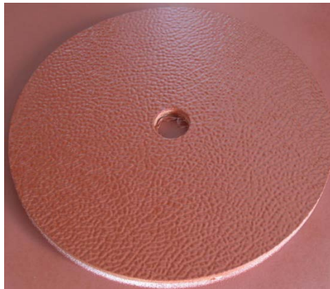
Figure 3.3. Picture of disk with high substrate roughness prior to coating application.
