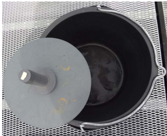
Figure 39A. System used to transport cylinder and prevent the sides from being touched. The upper left part was placed at the bottom of the bucket.
