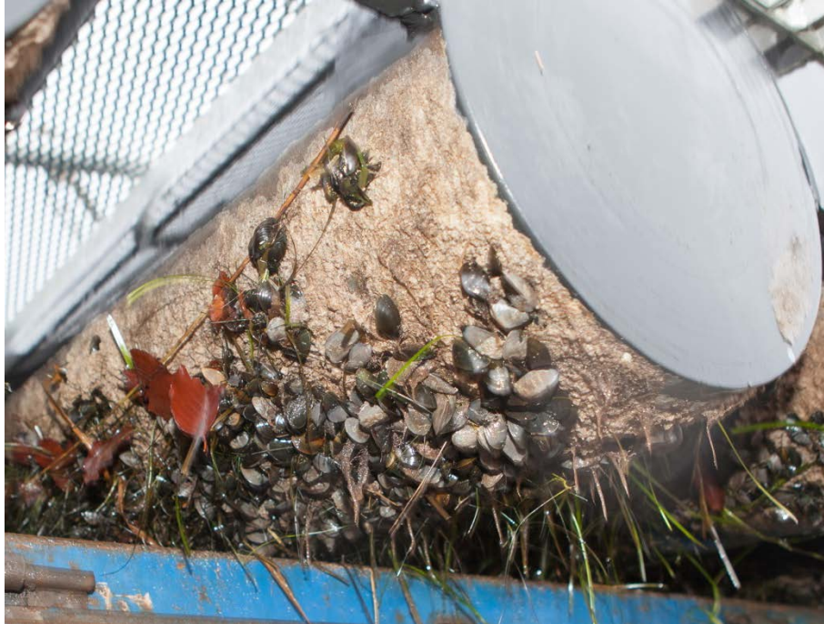
Figure 5.4. Close-up of the raft bottom after approximately 6 months of immersion in Roskilde Fjord. The end of the horizontal cylinder had been cleaned to show the PVC substrate.
