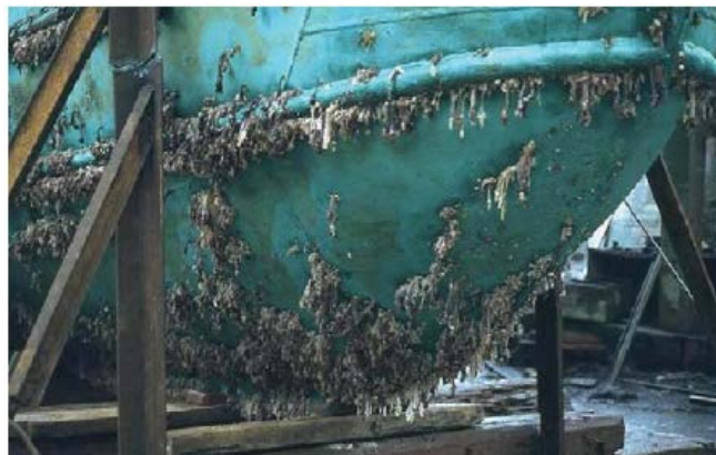
Figure 21.1. A hull with severe macro-fouling (Yebra et al., 2004). Reprinted with permission from Progress of Organic Coatings .
