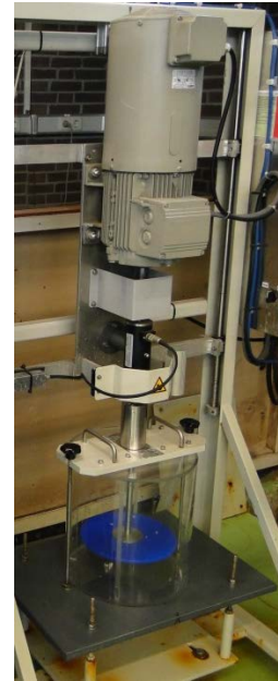
Figure 6.1. Friction disk machine at TNO, Den Helder (Klijnstra, 2014).
