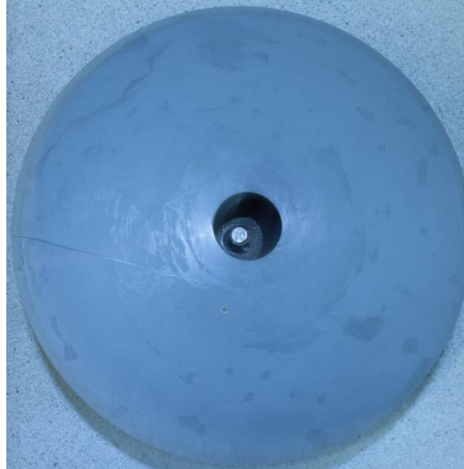
Figure 17A. Picture of the top and the inside of the smooth cylinder. The mounting system of the smooth cylinder works by turning the cylinder directly on to the shaft (no screw) and into the inner thread of the shaft.
