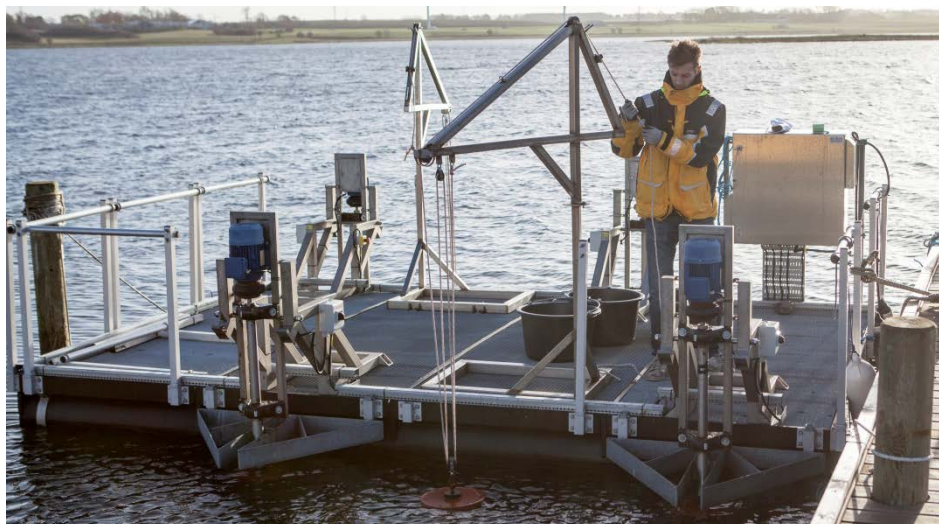
Figure 26A. Four cylinders exposed dynamically and two statically.
