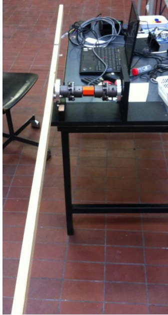
Figure 7A. Calibration setup where the torque sensor was retrieved from the shaft and mounted in a setup.
