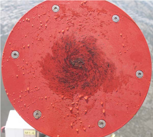
Figure 1.5. Biofouling pattern observed at bottom of cylinder.
