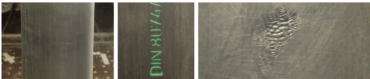
Figure 3. Cable section model superficial roughness, label and localized defects.
