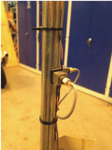
Fig. 6: Accelerometer mounting at the mid tower.
