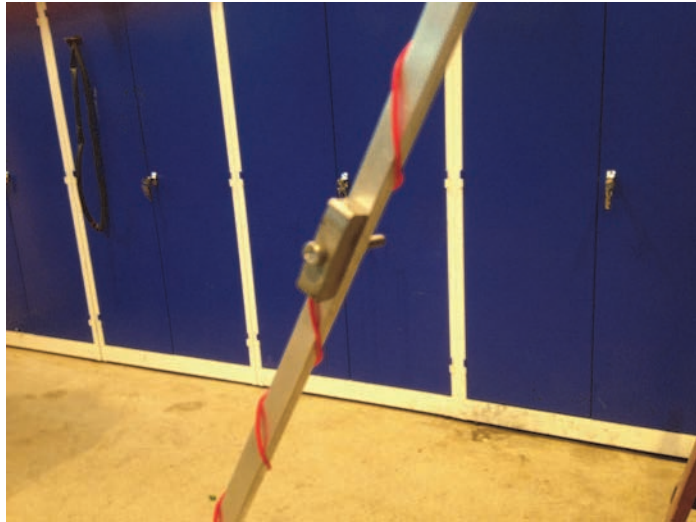
Fig. 5: A simple mount of an extra weight on one blade.
