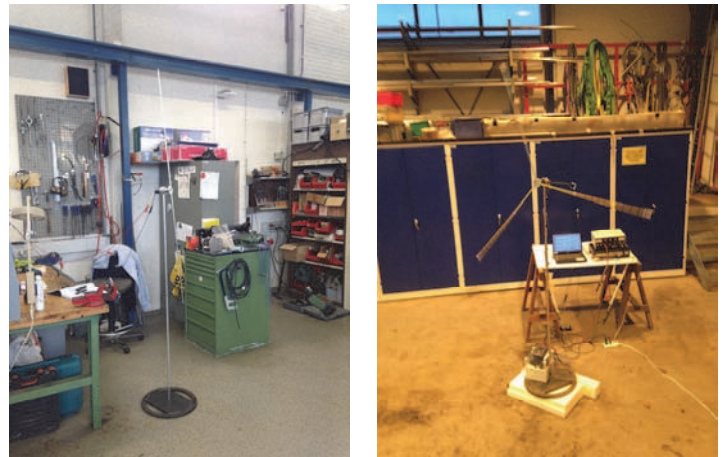
Fig. 3: Model turbine in two-bladed configuration (left) and three-bladed configuration (right).
