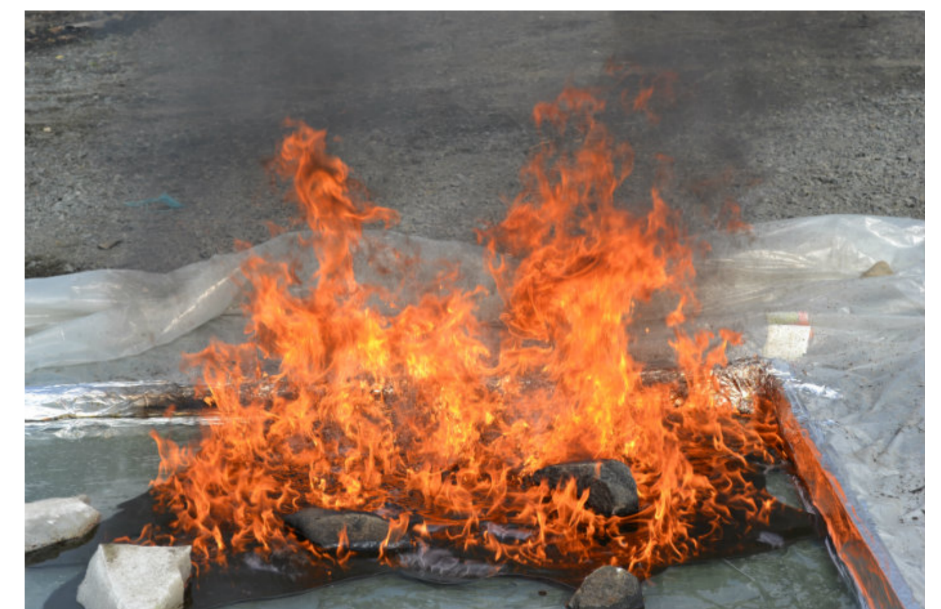
Photo 5. Oil burning in first burn
