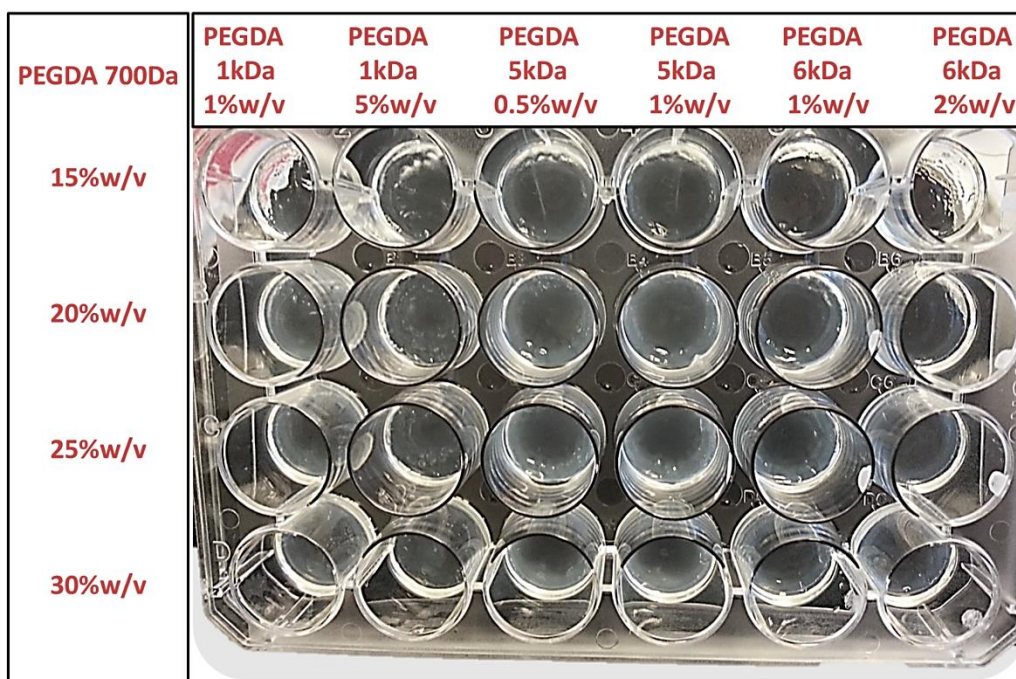
Figure 2.7 Hydrogel fabrication using 1%w/v IrgaCure 2959 dissolved in acetone/water (1:1). PEGDA (700Da) solutions are mixed with various concentrations of different PEGDA chain lengths (1kDa, 5kDa and 6kDa). Photo of a 24 well-microtiter plate where the mixed PEGDA compounds are exposed to UV-light for 1 h in presence of photoinitiator. Less colored and softer hydrogels are obtained when PEGDA 700Da is mixed with different PEG chain lengths, and all the tested amounts generate a crosslinked solution even though with some inhomogeneity.
