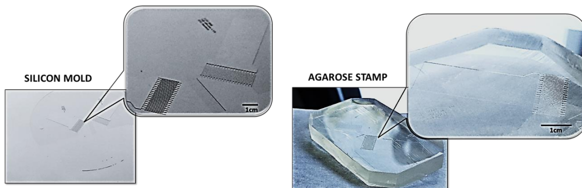
Figure 3.10 Photos of the main components required for printed dissolution procedure. On the left, the pictures indicate the silicon mold used for fabricating the agarose stamp. It contains two sets of inter-digitated electrodes 100µm wide and 100µm spacing. On the right, the agarose stamp produced by melting an agarose solution onto the silicon mold. After cooling down a negative replica of electrodes is obtained on the stamp surface.
