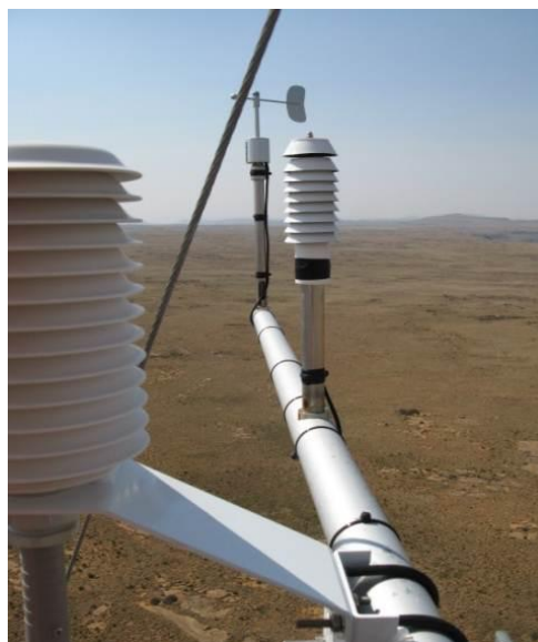
Figure 5. Wind vane, temperature gradient sensor and temperature/relative humidity sensor (foreground)
