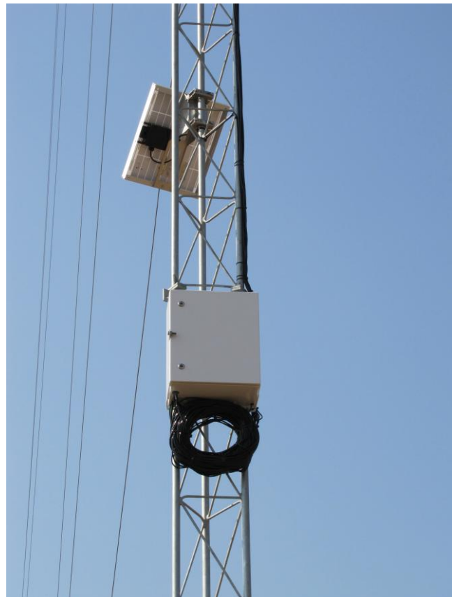
Figure 4a & 4b. Anemometer installation and data logger with solar panel (excess cable coiled below data logger housing)
