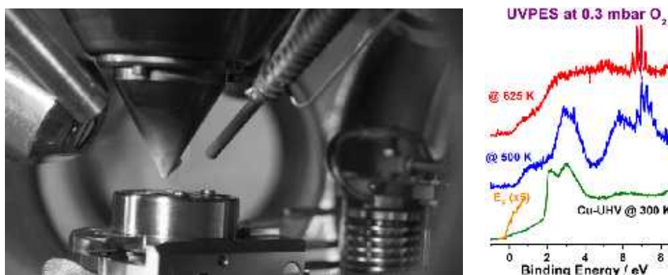
Figure 1: Open-reactor in NAPPES and Cu oxidation to \text{Cu}_2\text{O} and CuO.
