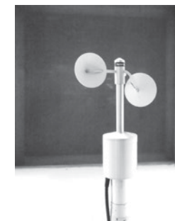
Fig. 1: Vector Instruments A100 LK cup anemometer calibrated at the IDR/UPM Institute after a service period on the field.
