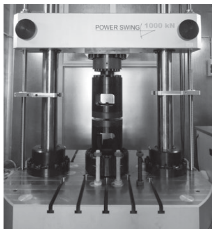
Fig. 1: Test set-up with bolts M36 at the TTH
