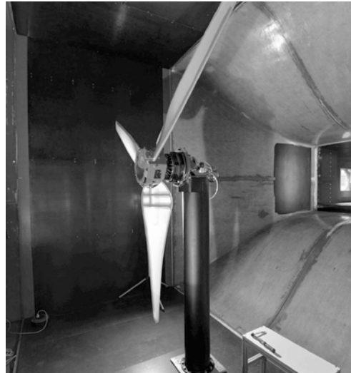
Fig. 1: The research wind turbine at the settling chamber of GroWiKa – TU Berlin
