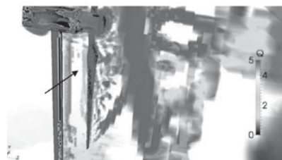
Fig. 1: Vortex structure in the wake of tower and blade of the downwind turbine simulation.
