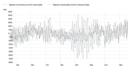
Fig. 2: Aeroelastic simulation of the flapwise bending moment
