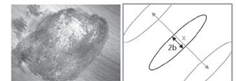
Fig. 3: Fretting damage and oscillatory movement in a blade bearing [2]
