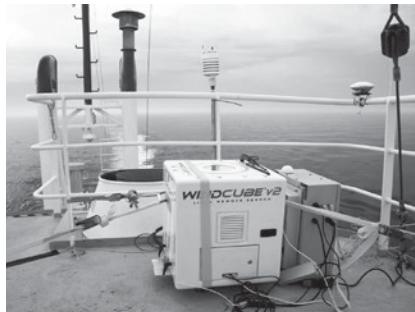
Fig. 1: Ship-lidar system installed on the top deck of the support vessel LEV Taifun.
