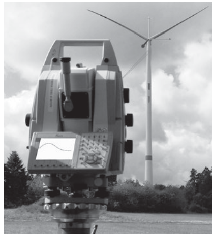
Fig. 1: scanning the profile at max chord
