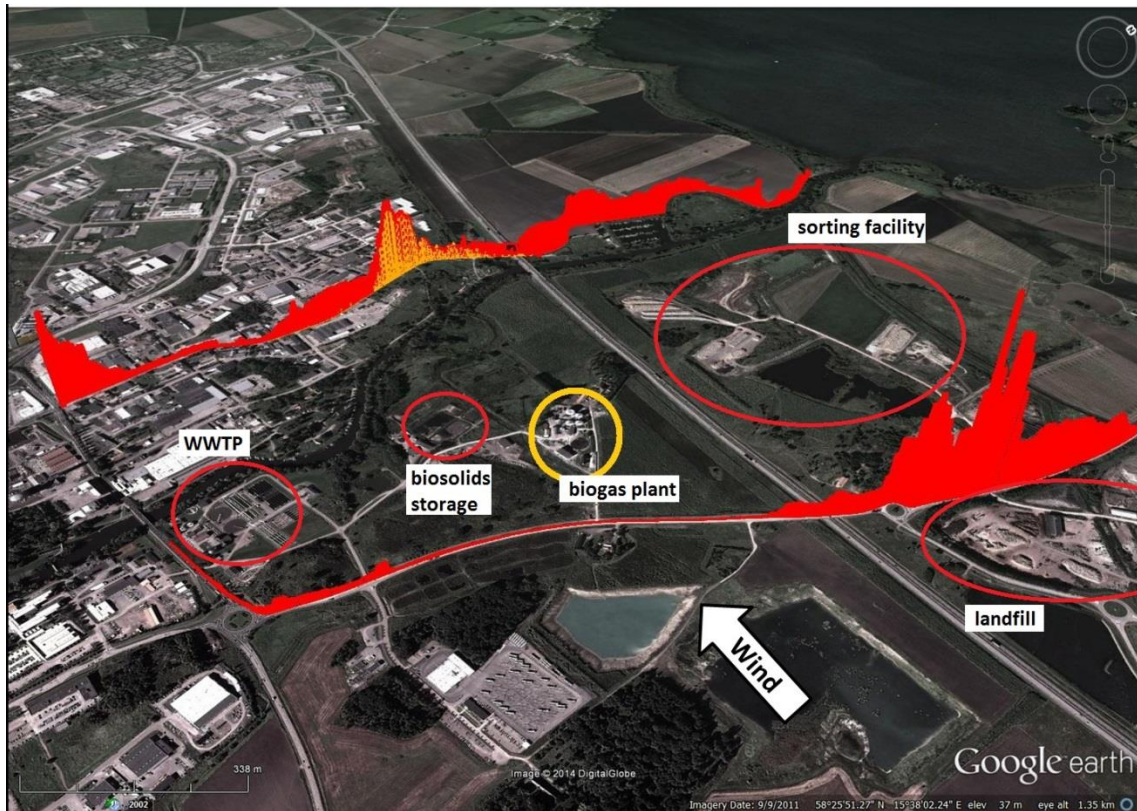
Figure 7. Methane screening of biogas plant surroundings with wind blowing from east.
