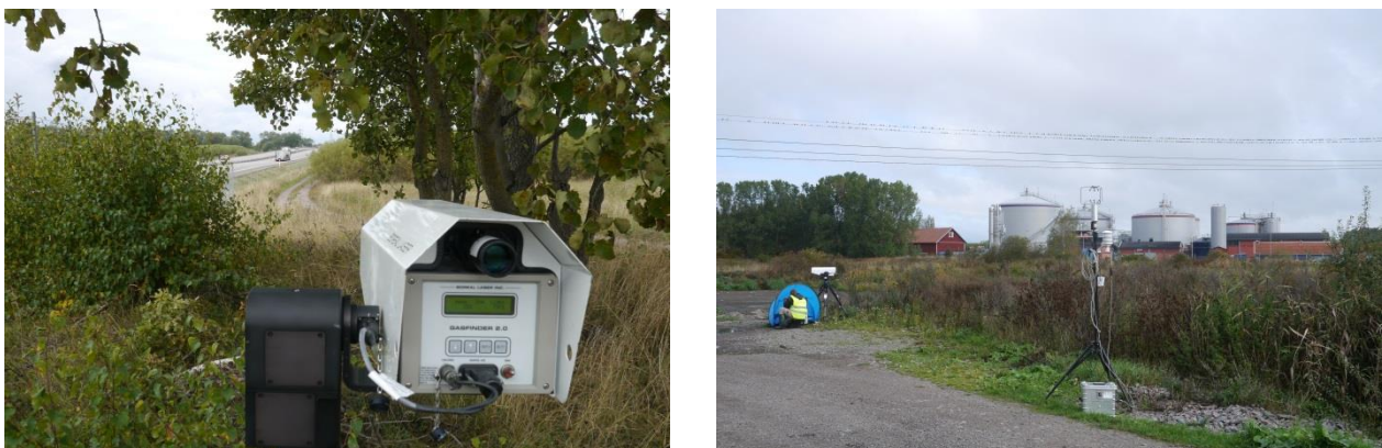
Figure 3-3-1: TDLAS back view (left) and in the downwind plume of the biogas plant together with the weather station (right). (Photos: DBFZ/Carsten Tilch)
