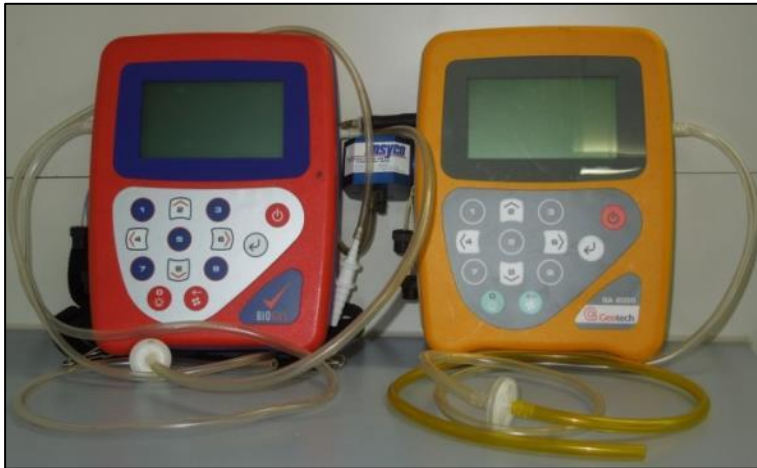
Figure 3: Available biogas monitors [DBFZ, Torsten Reinelt]
