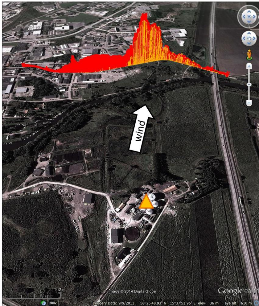
Figure 9. Atmospheric concentrations of methane and tracer gas above background level at approximately 900 meters downwind from the biogas plant measured on September 10th, 2014 at 17:34. The yellow triangle marks the placement of the C_2H_2 tracer gas release on the facility.
