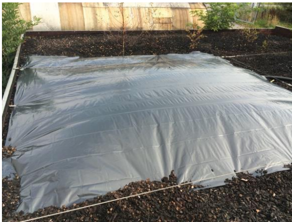
Figure 16. DBFZ sampling set-up at biofilter.
