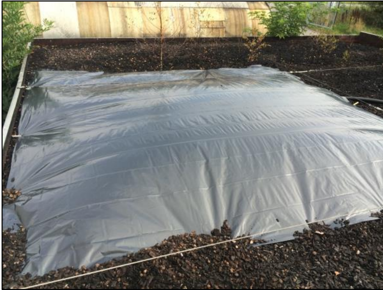
Figure 9: Measurement setup at an open biofilter
