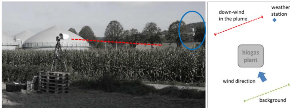
Figure 1. The setup of TDLAS for BLs modelling of the emission rate from area sources.
