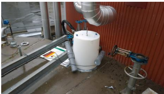
Figure 15. DBFZ sampling set-up at homogenization tank – hole.
