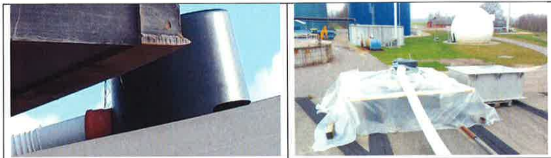
Figure 2. Different examples on design and designs of air suckling devices depending on type and area of methane leak. The air suckling devices has to be fitted to the shape and type of the leakage. The air suckling device shown left is involved with sampling of methane emission from single point leakage. The air suckling device shown to the right is designed for measurement of methane emission from a mixing pump cover situated above a digestion tank.
