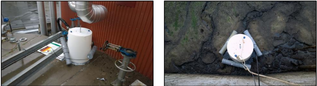
Figure 6: Use of the closed chamber (left: on a hole of the homogenization tank; right: on the surface of the open digestate storage)
