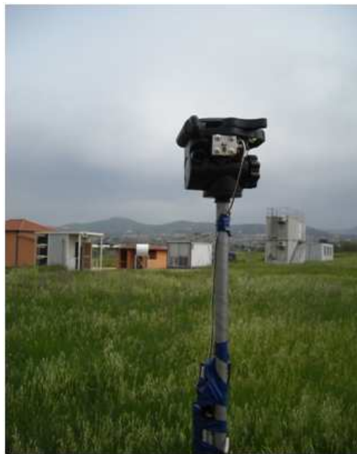
Figure 104. A recent maintenance intervention at the MTP5 radiometer – a microwave source for scanner alignment – (for courtesy concession of ISAC CNR Rome, Italy)
