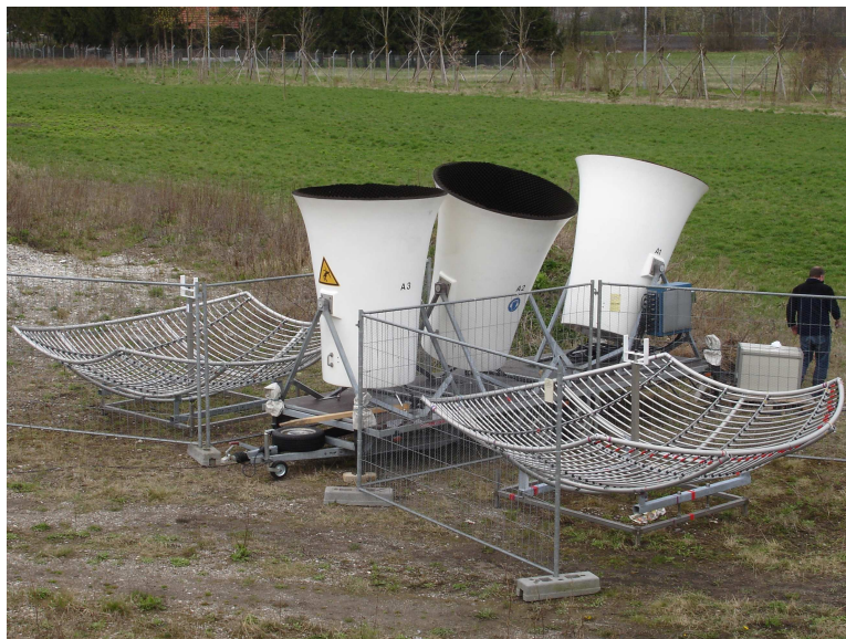
Figure 91. Sodar-RASS. The acoustic antenna is in the middle, the electro-magnetic antennas to the left and right.
