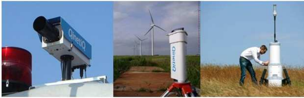
Figure 33. Stages of evolution of the ZephIR lidar. The left-hand picture shows the lidar head mounted on the nacelle of a Nordex N-90 wind turbine (March 2003). The central picture shows prototype ground-based wind profiler at Risø wind energy test site, Høvsøre, Denmark. The right-hand picture shows a ZephIR production model deployed in the field
