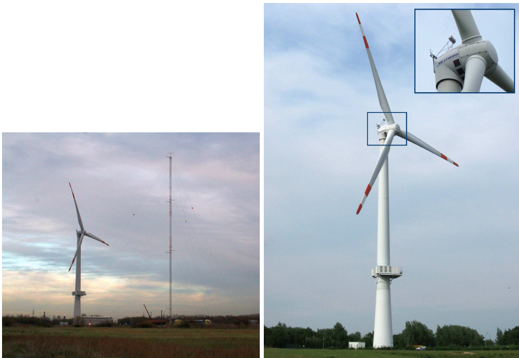
Figure 83: Onshore test site with AREVA M5000 and SWE met mast (102 m) (left) Installation of the LiDAR system on the nacelle of the turbine (approx. 105 m AGL) (right).
