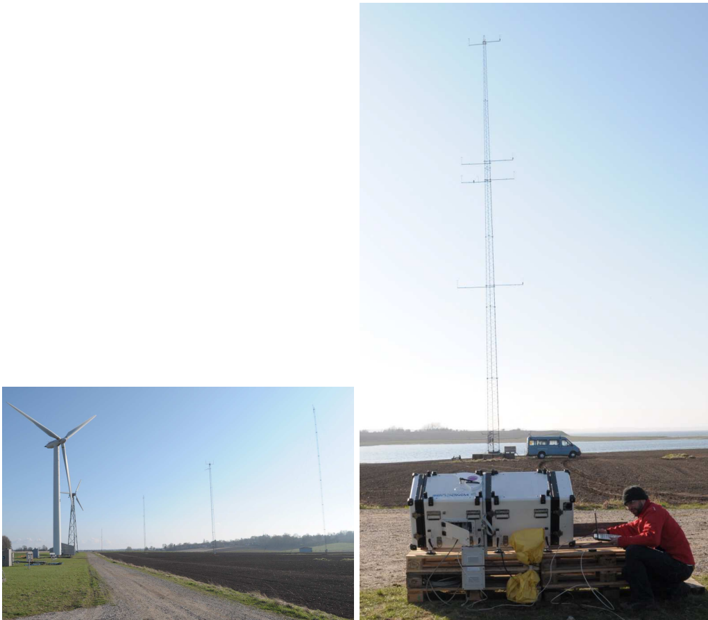
Figure 84: Test site at Risø-DTU with the Nordtank and Tellus wind turbines and several met masts (left). Tilted SWE LiDAR system pointing to a met mast (right).
