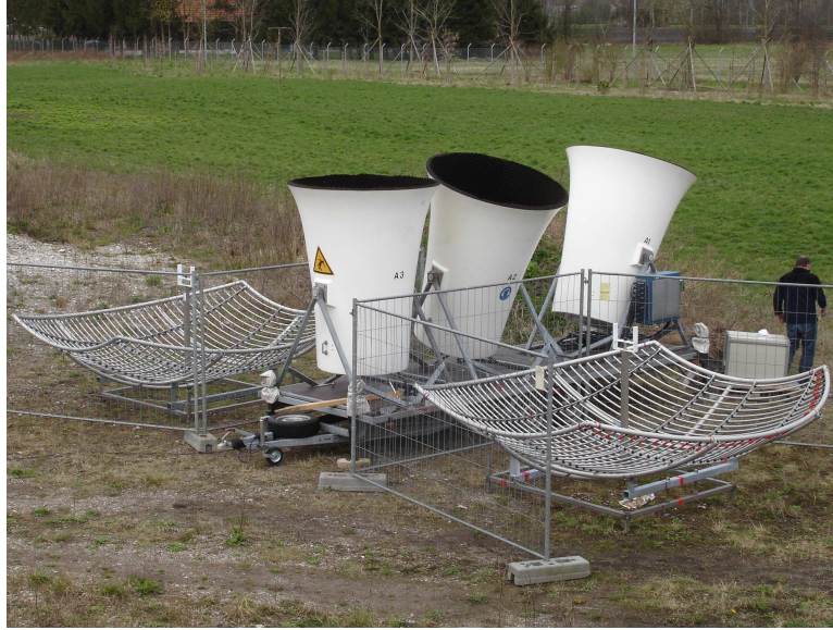
Figure 110: Sodar-RASS. The acoustic antenna is in the middle, the electro-magnetic antennas to the left and right.
