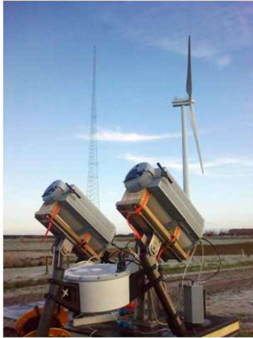
Figure 5: Two CW wind lidars belonging to the Windscanner.dk research facility being inter-compared and tested up against the tall meteorological masts at Høvsøre, Risø DTU.
