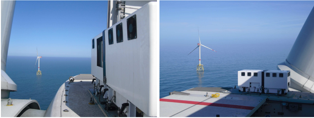
Figure 85: LiDAR system (scanner unit and Windcube) on the top of a Repower 5M measuring the inflow.
