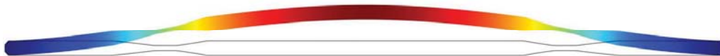
Figure 4. Optimized design for minimizing the cubic nonlinearity of a clamped-clamped beam and its linear vibration mode. The color in online version indicates the vibration amplitude.
