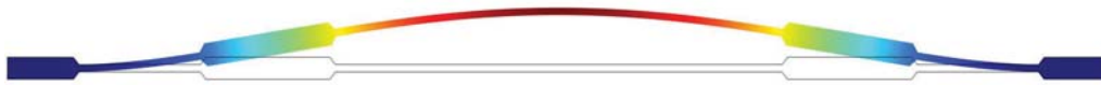
Figure 3. Optimized design for maximizing the cubic nonlinearity of a clamped-clamped beam and its linear vibration mode. The color in online version indicates the vibration amplitude.
