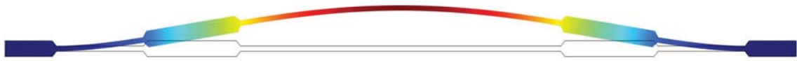
Figure 6.2 Optimized design for maximizing the cubic nonlinearity of a clamped-clamped beam and its linear vibration mode. The color represents the vibration amplitude. Figure taken from [P2].
