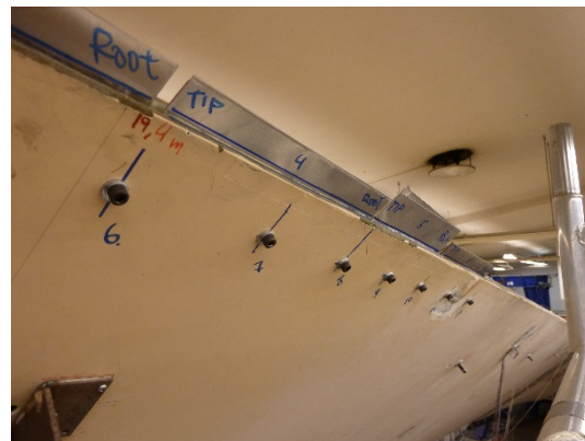
Figure 6. Bolts and metal plates used to change damage size in the second experiment.
