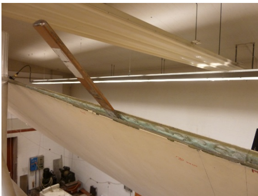
Figure 5. Blade damage in the trailing edge, with the chisel used to introduce the damage
