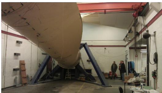
Figure 1. SSP34m blade mounted on the test rig
