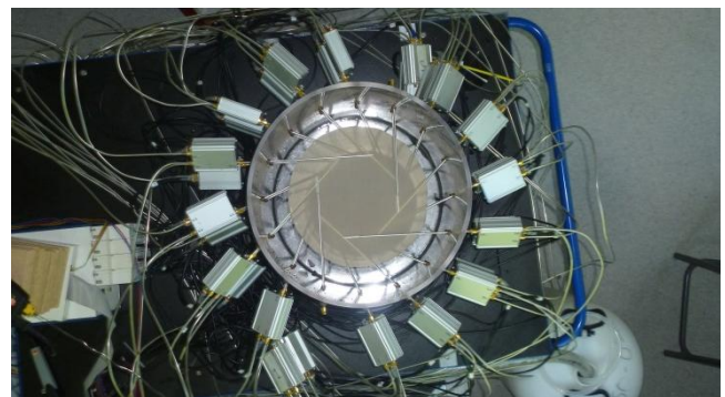
Fig.2. Top view of the tank with antennas and their data acquisition units.
