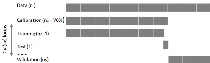
Figure 6.8: Schematics representation for LOOCV scheme used for calibration and validation of prediction of API concentration. Total samples, n = 75 . Modified from [167]
