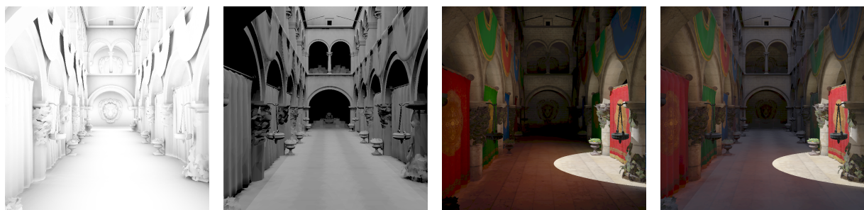
Figure 1: All images are generated using rasterization and layered depth maps. From left to right: Ambient obscurity, ambient occlusion, single-bounce indirect lighting, and environment lighting combined with indirect lighting.
