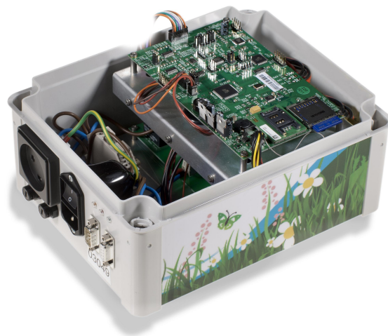
Figure A.1: Close up of the Smartbox with cover removed.
