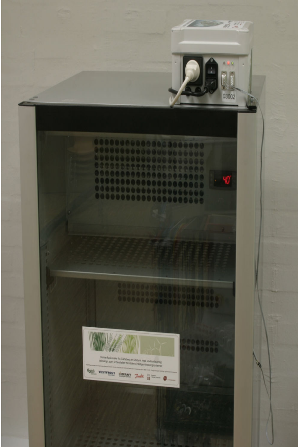
Figure 4. DFCR device placed on the top of refrigerator, with serial communication wire visible.
