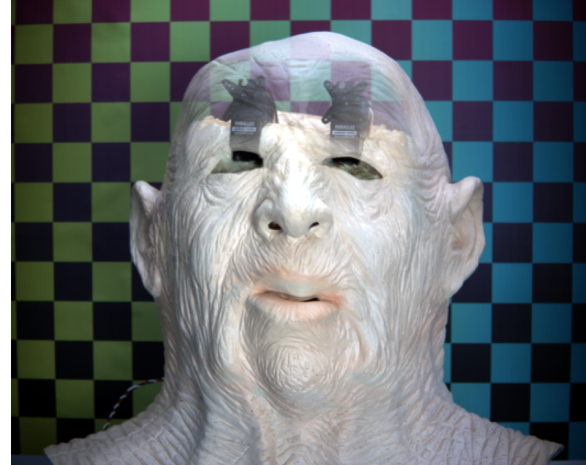
Figure 6. Actuators for manipulating the geometry of the mask. The image of the mask has been superimposed on an image of the actuators, illustrating their functionality.
