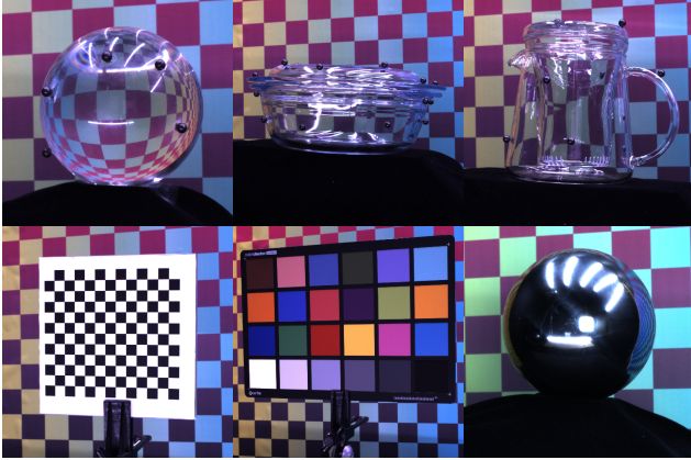
Figure 2. Preliminary images from our data set. In the first row, three glass objects (sphere, bowl, teapot) with markers placed on. On the second row, three calibration and rendering tools part of the pipeline: a black and white checkerboard (coordinate estimation), an X-Rite ColorChecker® (color balance compensation) and a chrome sphere (environment light evaluation).
