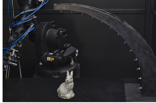
Figure 4. Capturing the BRDF of an object with known geometry. All illumination directions and view-directions are covered for each type material present on the object.
