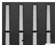
Cantilever coated with ~4µm PDLLA
