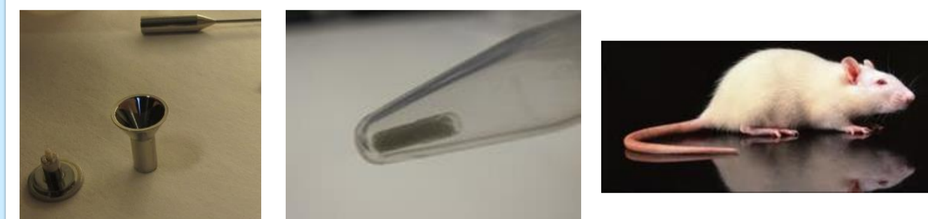
Fig. 3: Illustrations of the experimental methods. A) Fabrication of SU-8 microcontainers. B) Filling with drug powder (amorphous furosemide sodium salt). C) Spray coating of a lid of Eudragit® L100 or chitosan. D) In situ intestinal perfusion studies and oral bioavailability studies in rats of the drug-filled microcontainers coated with Eudragit® L100
