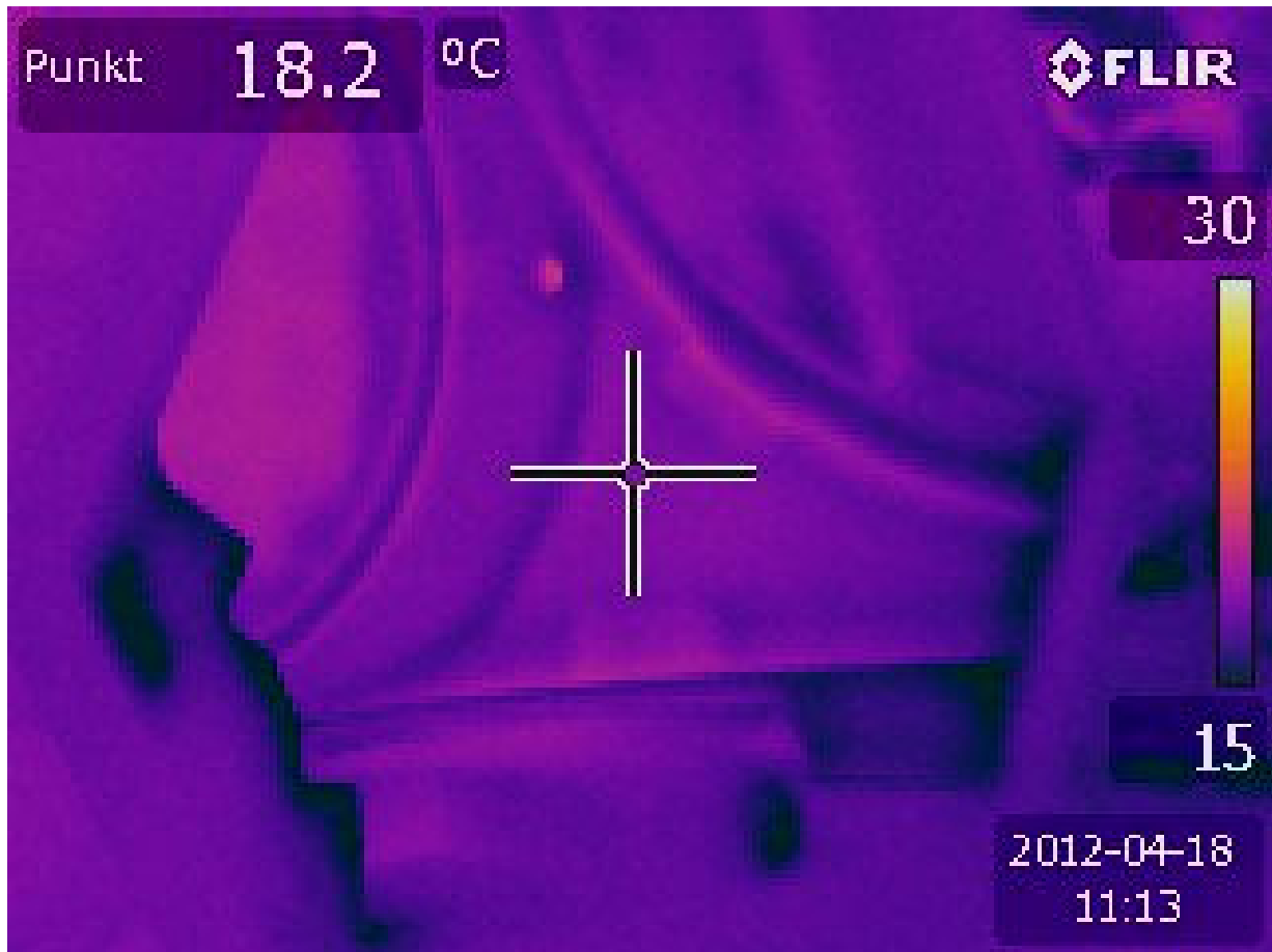
Figure 3.38 Thermography of a mould coated with water based coating. Cold spots can be identified as the last to dry and final moisture measurement performed.
