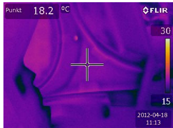
Figure 11. Thermography of a mould coated with water based coating. Cold spots can be identified as the last to dry and final moisture measurement performed.
