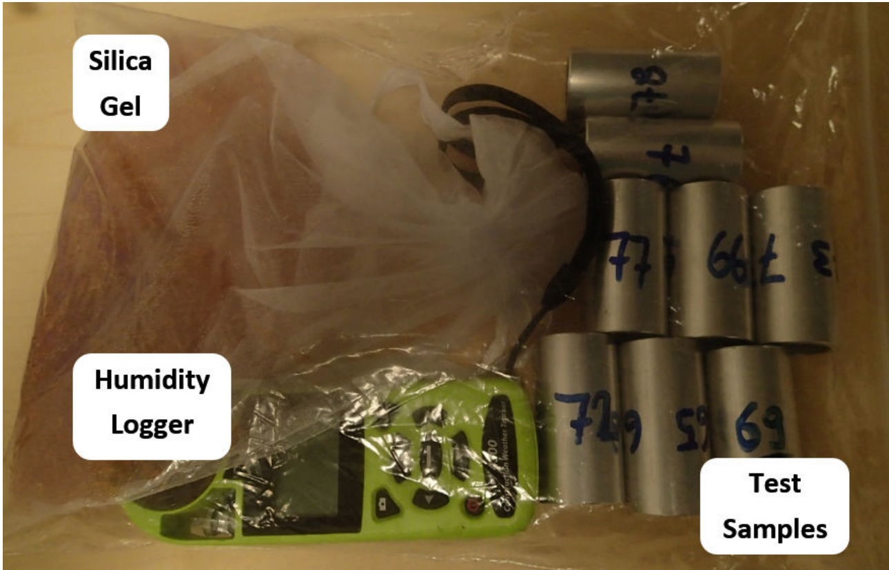
Figure 2.23 Equilibration of sand sample at 5-7% RH before moisture adsorption diffusion tests.
