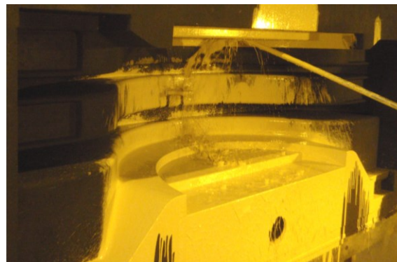
Fig. 1: Furan sand mould coated with water based foundry coating.
