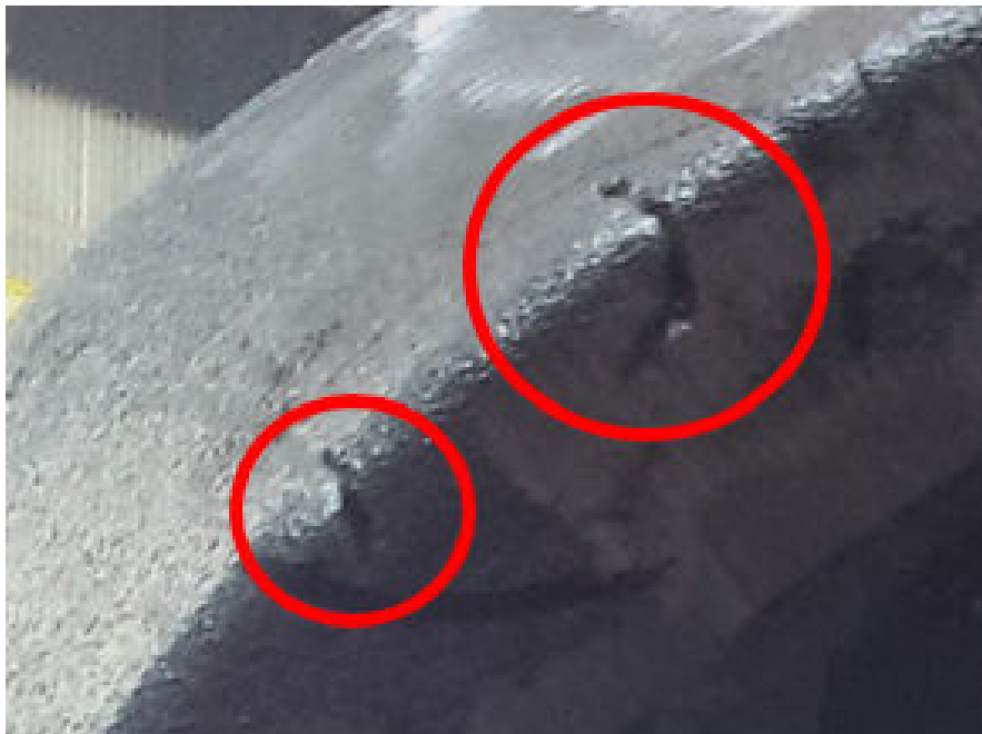
Figure 1.8 Example of moisture related casting defect,
