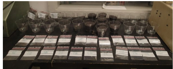
Fig. 10. Sand from two different factories is sieved according to factory standard to eliminate dust and fines.
