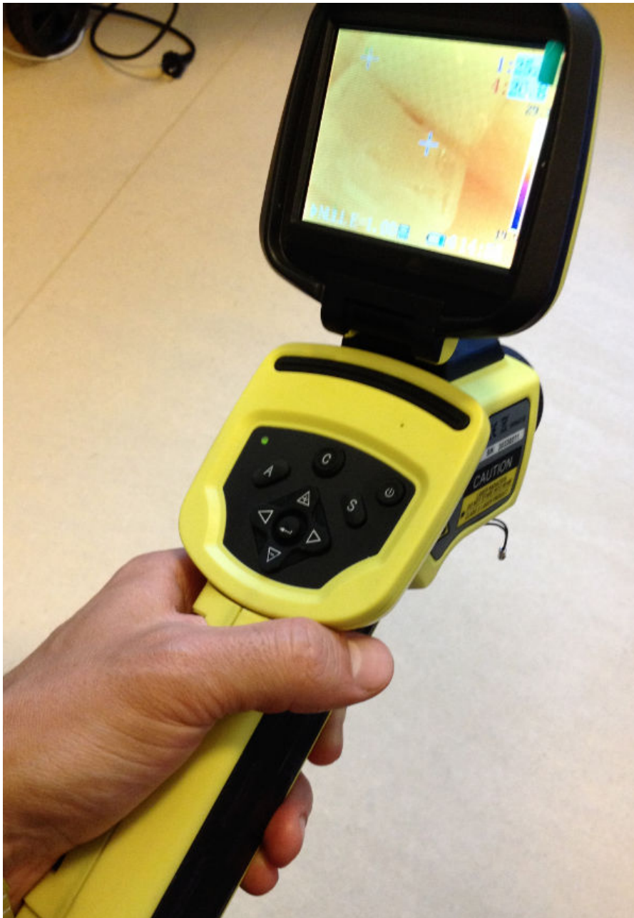
Figure 2.31 Infrared camera for temperature surface measurement in large moulds.
