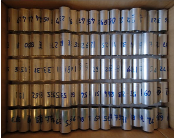
Fig. 16. Samples drying in natural air at 25°C and 50% relative humidity for 1 week.
