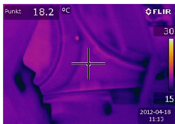
Figure 9. Hub mould surface temperature measurement done with infrared camera. Areas near corners have lower temperatures due to lower heat exchange coefficient as shown by simulation.
