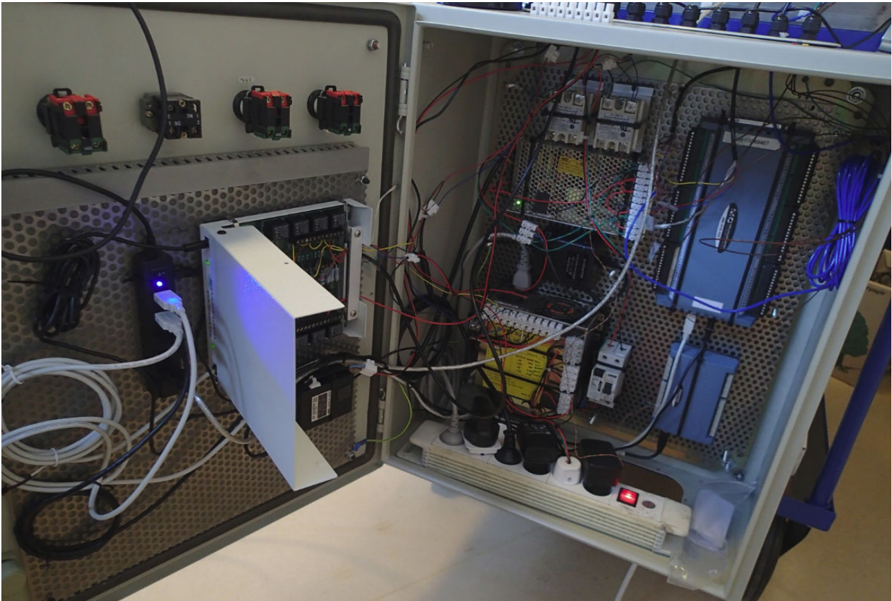
Figure 2.14 Picture of acquisition cards and power supplies for the experimental drying setup.
