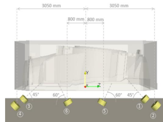
Figure 10. Optimal fan arrangement for main foundation mould.
