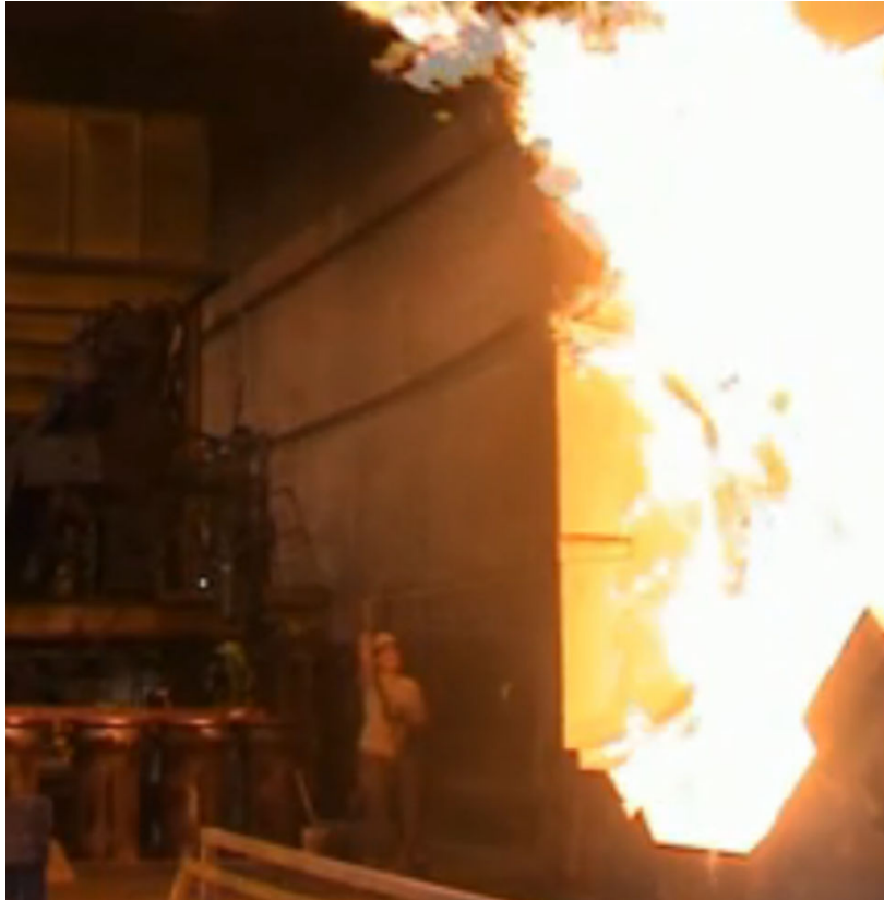
Figure 1.2 Drying of alcohol based coated mould generating 6 m high flames (on the right), and operator standing nearby (on the left).
