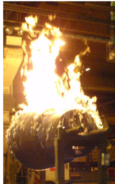
Figure 1. Drying by burning of core coated with alcohol based foundry coating.
