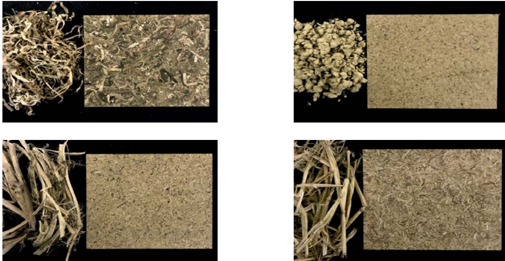
Figure 1: Different bio-based building products created in a project at the Danish Technological Institute [4]. Top left: Eelgrass, Top Right: Seaweed waste, Bottom left: Tomato stems, Bottom right: Straw
