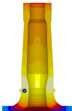
Figure 7. Contour plot of the temperatures on the cross section of the main shaft, and the point where the temperature curves are extracted.
